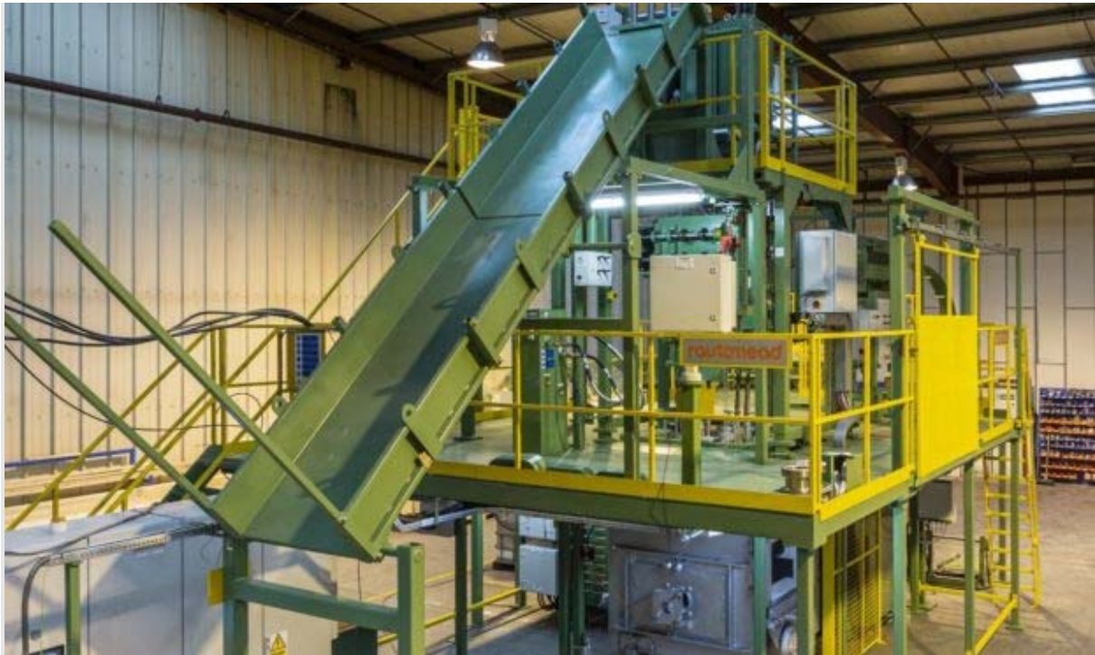
Rautomead's continuous casting machine.
